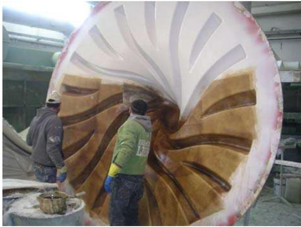
Impeller dia. 2700 under construction
